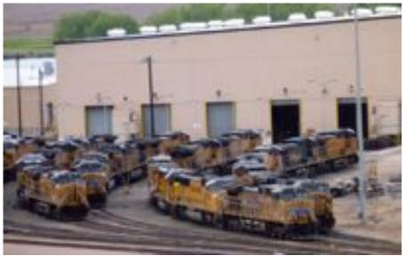
Each track in the huge engine house is several car lengths long within the building. Since regulations prevent live locomotives from entering the shop, the engineer must put together a string of engines (often six or seven other locomotives) before he/she picks up the locomotive needing service and then moves it to the rear of the facility. This activity necessitates a lot of switching to get the intended locomotive into the correct stall.
