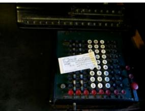
Above the scale ticket sits on a mechanical calculator that was extremely popular up until the advent of the electronics. These were common throughout industry well into the mid 1970's. Texas Instruments brought out their first electronic calculator in 1967. The pocket sized HP - 35
